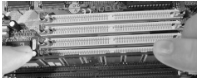
DIMM Modules are easy to install because the keyed sockets only allow the modules to be placed in one way removing the possibility of them being inserted in backward (unless you use a hammer).
