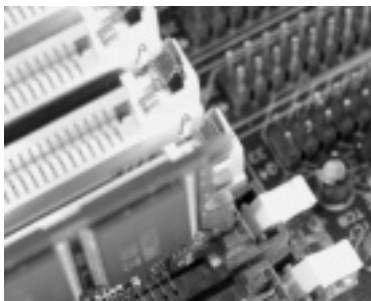
DIMM Modules are easy to install because the keyed sockets only allow the modules to be placed in one way removing the possibility of them being inserted in backward (unless you use a hammer).
